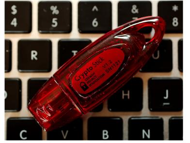
The GPF Crypto Stick is a USB stick in a small form factor containing an integrated OpenPGP smart card to allow easy and high-secure encryption e.g. of e-mail or for authentication in network environments.
